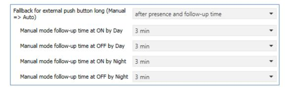
The follow-up time can be set as desired. Now connect object 4 - external push-button long (for light channel 1) to the push-button which is to **switch-Off** the light.
